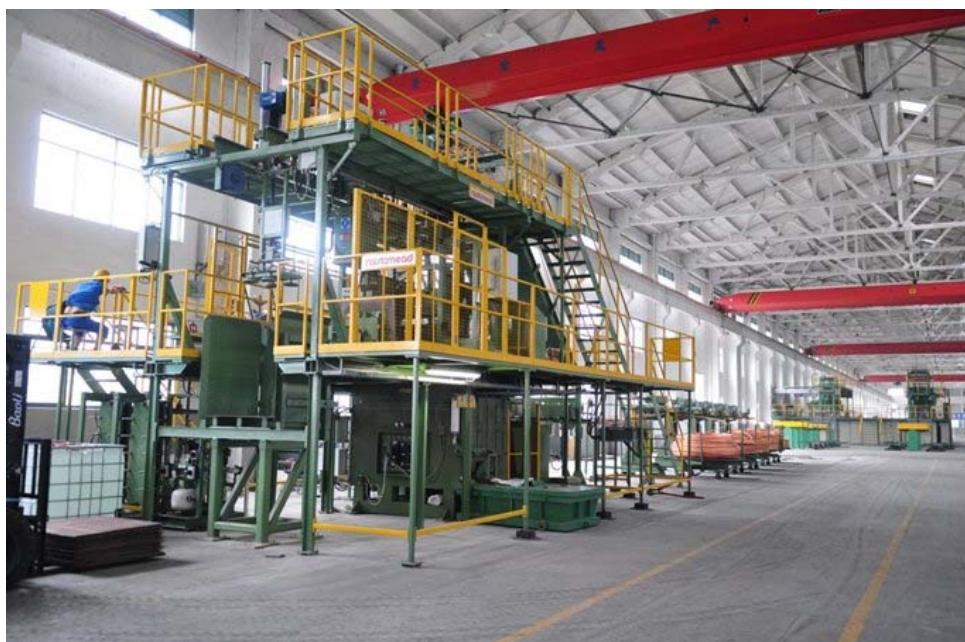
Fig. 9 Rautomead RS 3000/5-Cu-Mg Casting Machine
