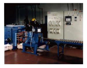
Fig 3 Horizontal continuous casting of gold strip for Kruggerand production in South Africa
