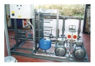
Fig 10 Primary water cooling module
