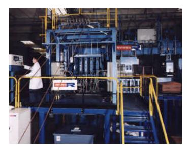
Fig 15 Model RS 2300/4/30 in production of 19mm diameter rod in CuMg0.35
