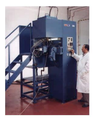
Fig 4 Production of gold rod for fine drawing to bonding wire
