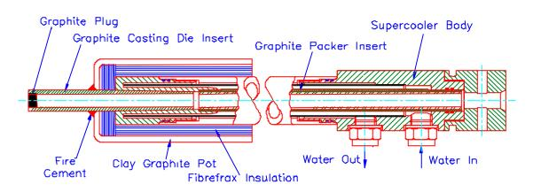
Fig 7 Casting Die assembly
