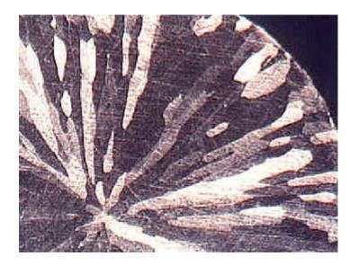
Fig 14 Magnified photomicrograph of grain boundary area
