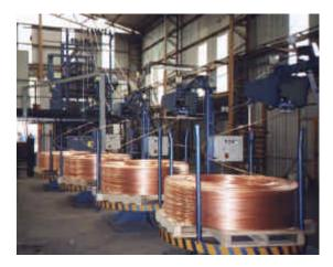
Fig 9 Rod Coilers
