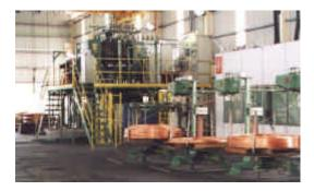
Fig 5 Model RS 3000/8/8 in production of Cu-OF at 8mm diameter
