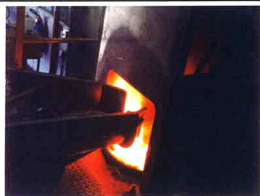
Fig 4 Vibrating Table feeding Swarf into Furnace
